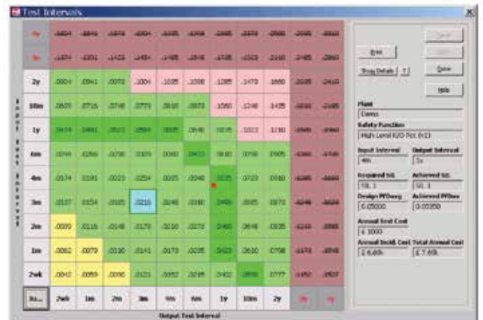
Test interval results are displayed graphically and issued via a comprehensive report with fully traceable and archived decision processes.
