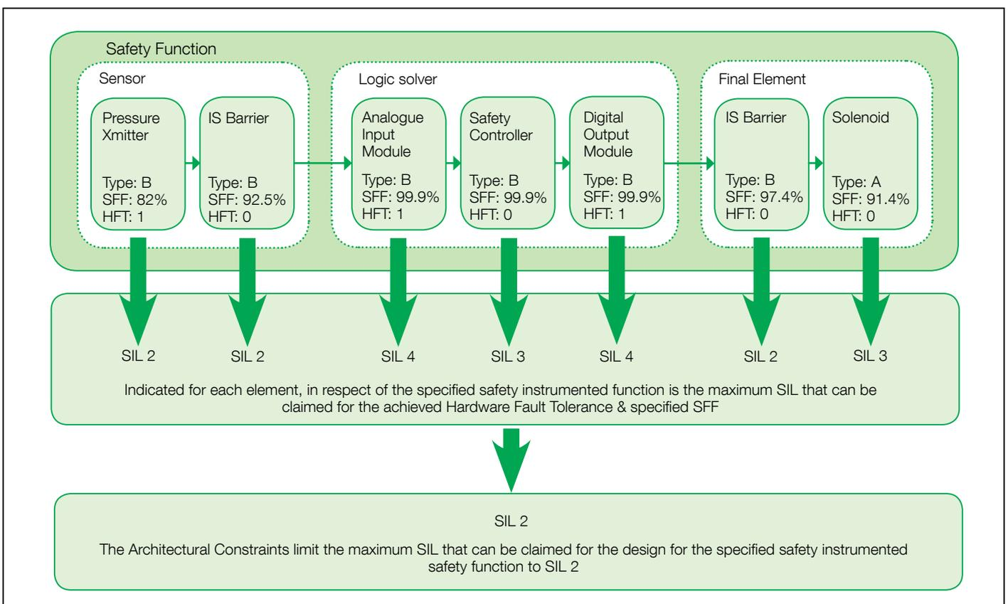
As can be seen from the example on page 18, the architectural constraint has been calculated for each element of the safety function. The architectural constraint is limited by the lowest achieved SIL (in terms of architectural constraint), the Final Element IS Barrier, which is limited to SIL 2.
