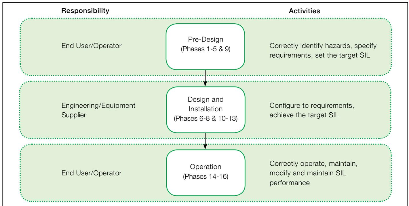
It can be seen from the diagram above, that each organisation has a responsibility to implement processes and to deliver packages of work to the next organisation in the supply chain. For example, the End User or Operator has a responsibility to provide sufficient information to the Engineering/Equipment Supplier to allow them to complete the design stage of the safety lifecycle.
